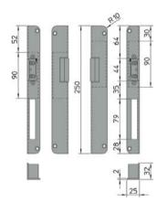
.1 for doors: RH opening inwards – LH opening outwards .2 for doors: RH opening outwards – LH opening inwards
