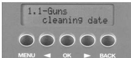
This function can be used to set an estimated date for the next gun cleaning.
