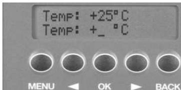
Enter the temperature in the two-digit format. If the internal temperature is 7 degrees, enter 07.
