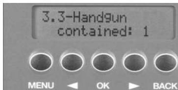
Press **OK**, enter the number of handguns contained in the cabinet and press **OK**. The new number will be memorized.
