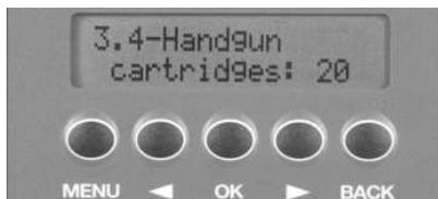
Press **OK**, enter the number of handgun cartridges contained in the cabinet and press **OK**. The new number will be memorized.
