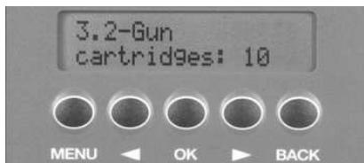
Press **OK**, enter the number of cartridges contained in the cabinet and press **OK**. The new number will be memorized.
