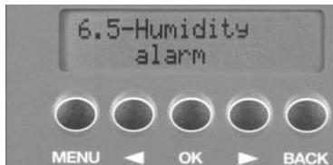
This function can be used to activate the alarm for too high humidity. This function is useful when the gun cabinet contains weapons, cartridges or objects that can be ruined by humidity and oxidation.
