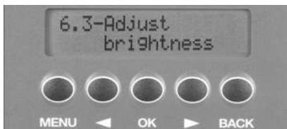
This function can be used to adjust the brightness of the display, to better adapt it to the lighting conditions of the room where the gun cabinet is installed.
