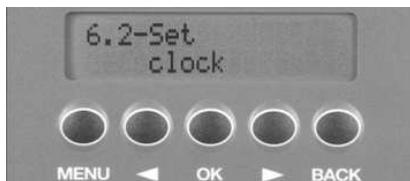
This function can be used to set the internal clock of the gun cabinet. Press **OK**. Enter the current time in the format 'hours:minutes'. Each entry must consist of two digits, so if the time is 7 minutes past 7, enter 07:07. The time format is from 00 to 24, so if it is 5 o'clock in the afternoon, enter 17:00.
