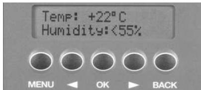
The temperature sensor can be calibrated by means of menu 6.7 (see page 33). The temperature has a precision of +/- 1°C, while the relative humidity is measured from 55% to 90% in steps of 5%.
