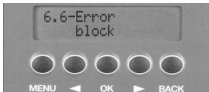
This function can be used to deactivate or set the duration of the time block after 6 consecutive code errors.
