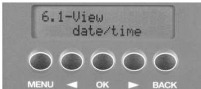
This menu can be used to display the current date/time in order to check that the internal clock is correct.
