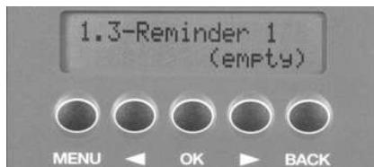
This function can be used to enter a **reminder/free text message, which will then be displayed every time the door is opened starting from the set date**. Up to 4 text message reminders can be entered (Menu 1.3, 1.4, 1.5, 1.6). If no reminder has been entered in the selected position, the second line of the display will show the message "(empty)"; otherwise the reminder and the set date will scroll across the display.
