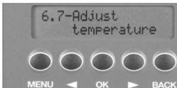
This function can be used for precise adjustment of the internal temperature sensor. It is first necessary to obtain the exact temperature inside the gun cabinet (e.g. by leaving a thermometer inside the gun cabinet for at least an hour).
