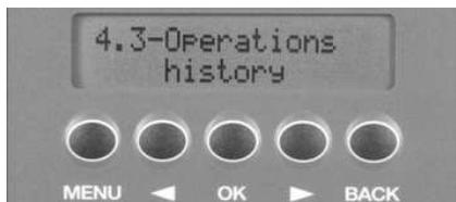
This function can be used to display the operations history of the last 50 operations performed on the gun cabinet.
