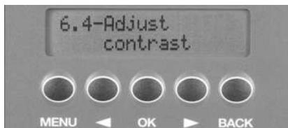
This function can be used to adjust the contrast of the messages on the display, to better adapt it to the lighting conditions of the room where the gun cabinet is installed.
