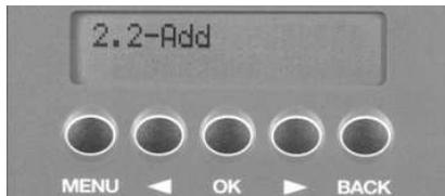
This function can be used to add the hunted quantities to the internal operations history. Press **OK**, use the **<** and **>** keys to select the species to be increased in quantity and press **OK**.
