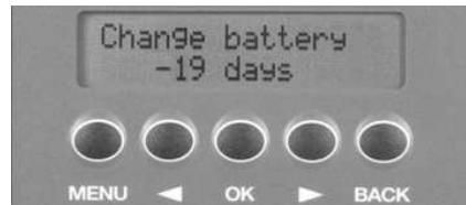
When the battery level is so low that correct functioning cannot be ensured, the following message will be displayed:
